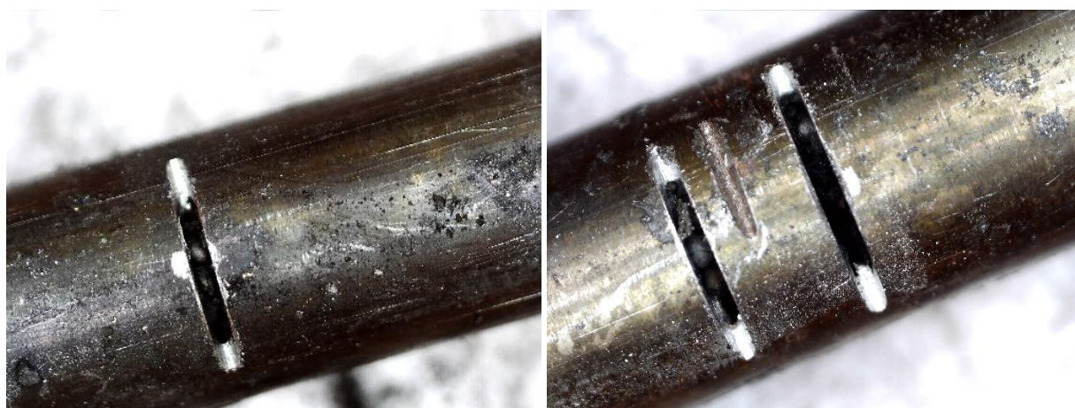
Figure 7 Images of first two cuts of MARINE pin 2, to allow fixing the sphere-pac fuel with resin.
