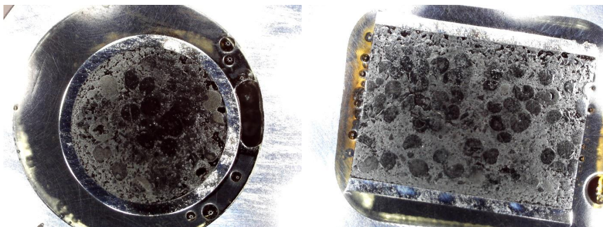
Figure 8 Impression of a prepared radial and axial specimen from pin 2.
