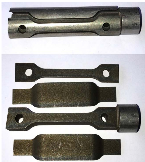
Figure 2. Uniaxial test sample extraction from cold worked bar by EDM
