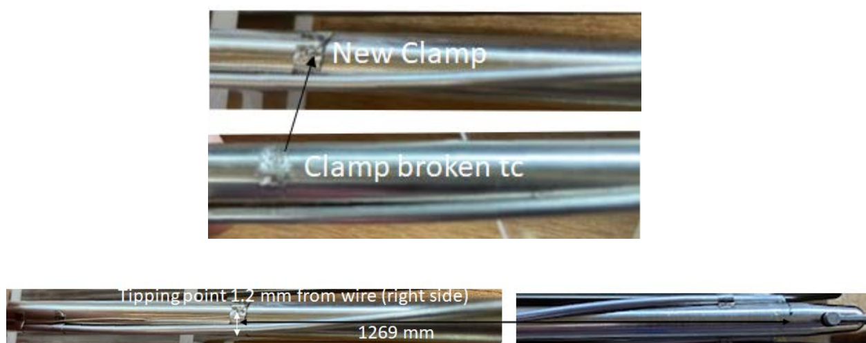
Fig. 8. Pin 5 Multi-point thermocouple and multi-diameter thermocouple tipping point.
