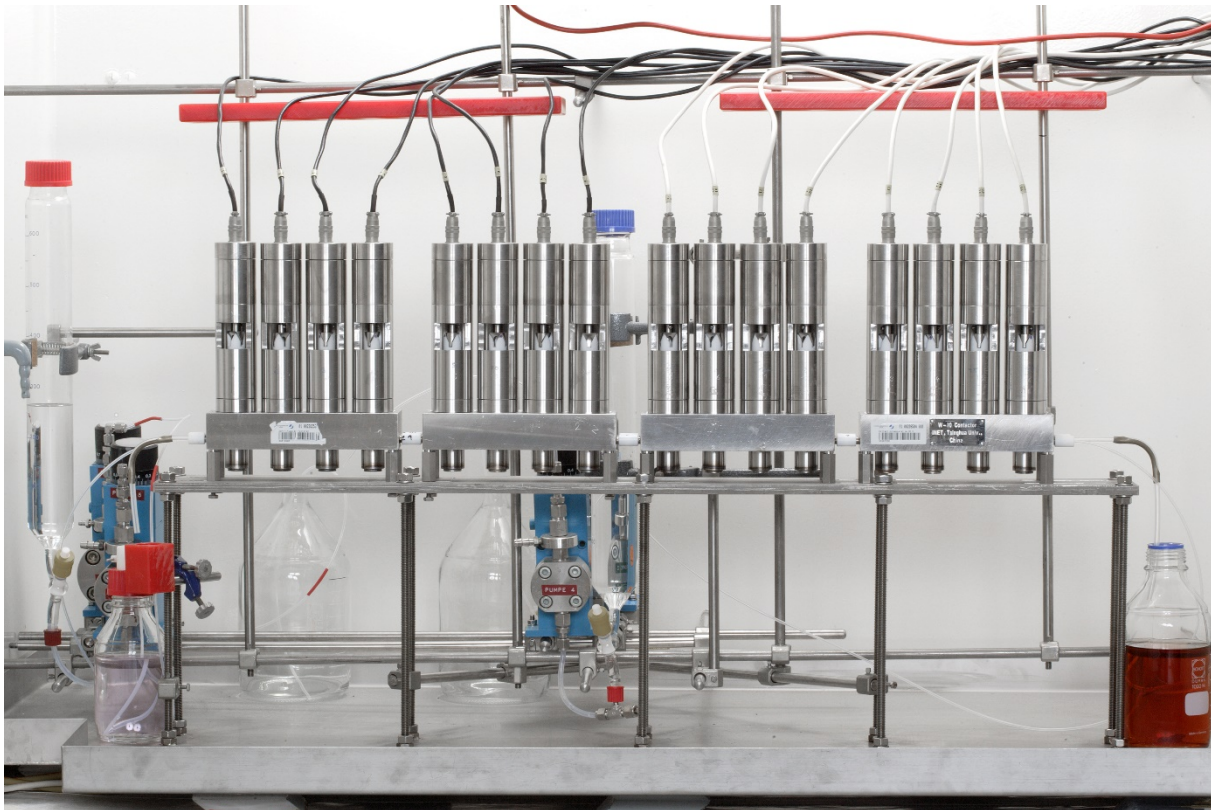
Figure 2 Centrifugal contractor cascade for spiked tests of flowsheets at Forschungszentrum Jülich research centre, Germany
