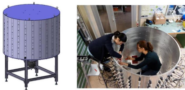
CERN 144:1 cavity combiner 144 kW CW @ 200 MHz calculations by ESRF within CRISP, construction by CERN
